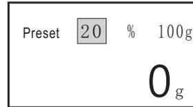
he first step of tension adjust: Press "√" button once, the cursor move to the number of percentage. Press "+" or "-" to adjust the first step of tension in term of percentage. 0 to 100 with respect to the minimum tension to maximum tension (The first step of tension is default when the tensioner is switching
