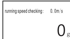
Wire running speed checking: A long pressed of "-" button to enter the speed checking interface. One more long pressed "-" to exit.
