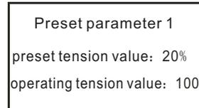
A long pressed "√" button in operation interface to enter the "preset parameter 1" page. The preset tension value (First step tension) and operating tension value (second step tension) can be set. Press "+" button to enter the "preset parameter 2" page or press "X" button to back to the operation interface if no adjustment is required.
