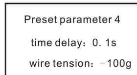
Press "√" button, to set the time delay (the time between the first step tension switches to second step tension. Not necessary to set usually) And the broken wire tension value (broken wire status is defined if the tension value shown is less than this value). Save and press "+" button to enter the "preset parameter 5" page.
