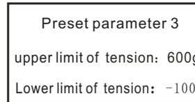
Press "√" button, to set the upper and lower limit of operating tension value (second step tension). When the tension value exceeds this limit set, the indicator light flash will flash and output an alarm signal. Save and press "+" button to enter the "preset parameter 4" page.
