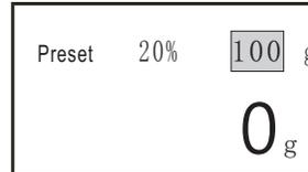
step of tension adjust: Press "√" again after setting the first step of tension, the cursor will move to the number with "g" unit. Press "+" or "-" to the required tension value, and press "√" to save and exit. (Signal toggle is required for 2nd step of tension)
