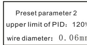
Press "√" button, to adjust the upper limit of PID (It is not necessary to tune because it can be adjusted automatically) and the wire diameter. Save and press "+" button to enter the "preset parameter 3" page.
