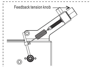
Rotate the feedback tension knob to adjust the back tension.
